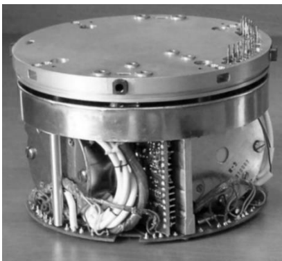
Fig. 2. Three-axis laser gyro with the body cover removed.
