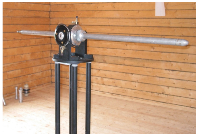
Fig. 4. Appearance of the calibration installation for inclinometers
