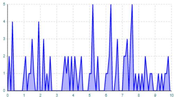
Fig. 4. Timing diagram of the FiFoSC5 operation drive: along the X-axis - model time, along the Y-axis - the depth of the drive memory filling.
